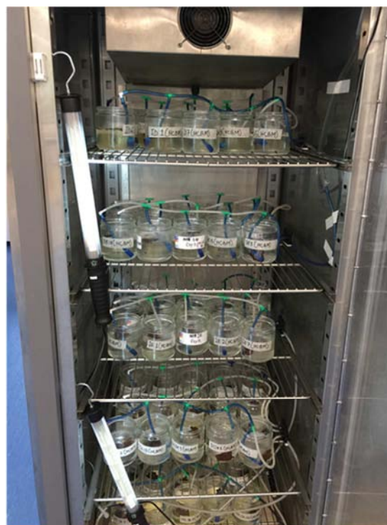
Figure 2. One of the experimental set-ups in the incubators showing the arrangement of the jars with one A. aquaticus in each jar exposed to experimental media (Solvent control (SCTR), Low treatment (LT) & High treatment (HT)).
